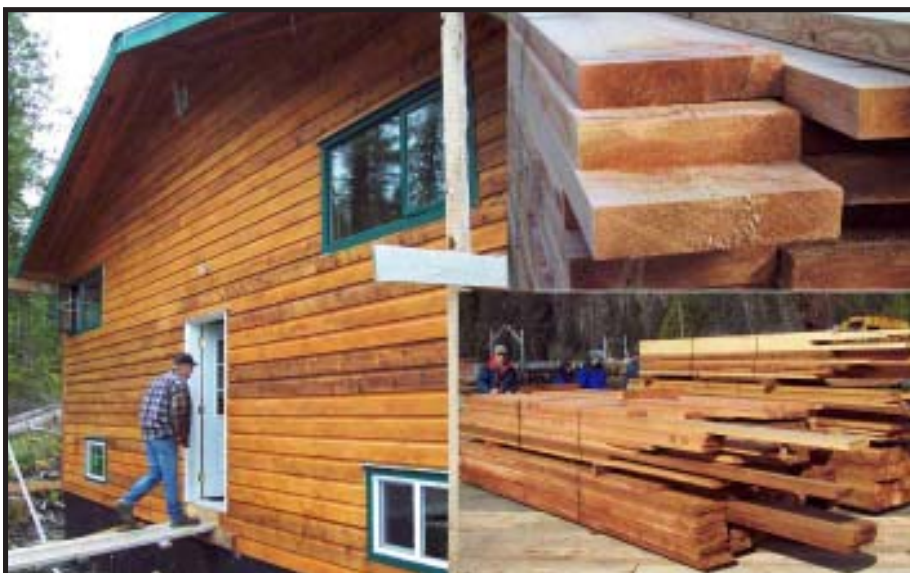
Figure 11. Some of the high quality redcedar siding and dimensional lumber produced at the Group Mills operation at Oona River.
