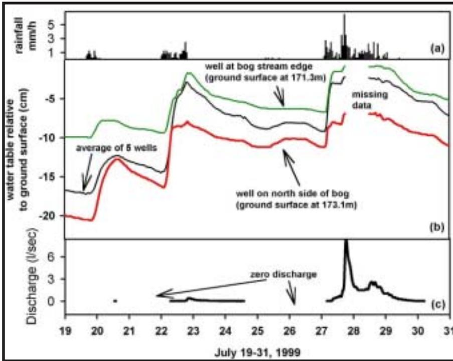
**Figure 4.** (a) Precipitation; (b) bog water table elevation relative to ground surface; and (c) discharge recorded at the bog weir.
