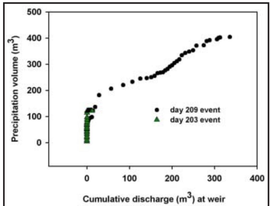
**Figure 5.** Cumulative weir discharge plotted against total precipitation volume. Each triangle (event 203) or dot (event 209) represents one hour. Note the vertical rise in precipitation volume for event 203 with no discharge change until very end of the storm. Most of the rainfall in the day 203 event is taken up by groundwater storage.
